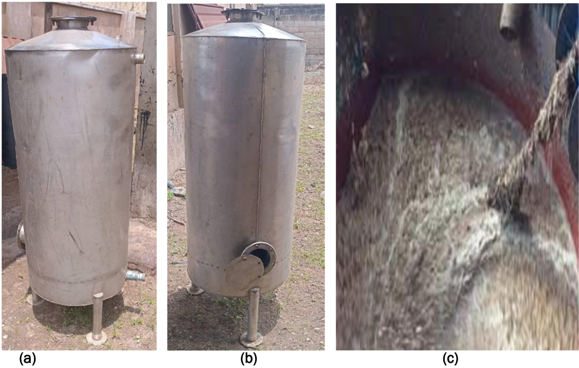
Plate 3.1 (a) and (b) Plate of the digester (c) Slurry from digester
