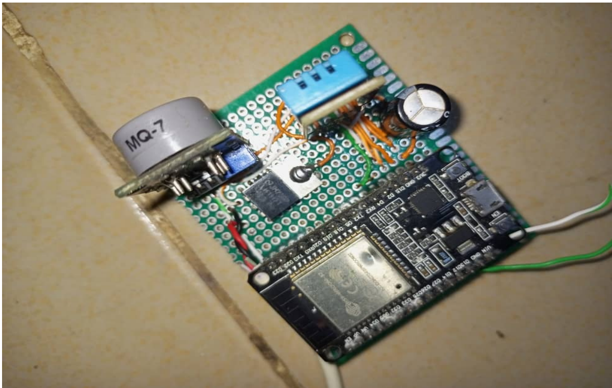
Figure 2.0a the developed Air quality monitoring device
