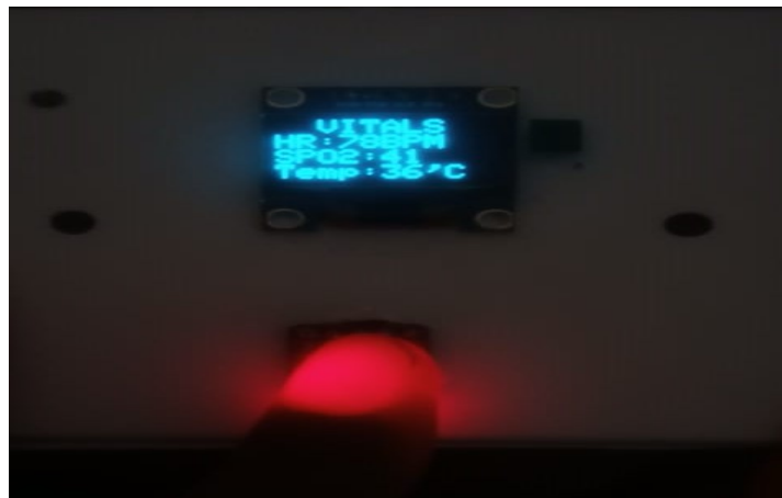
Fig.4.0d: Touching the OLED screen displays the user's vitals.
