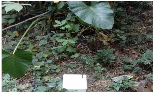
Figure 10: GSM based data acquisition system logging data at umuomaku in Orumba south local government area of Anambra state.
