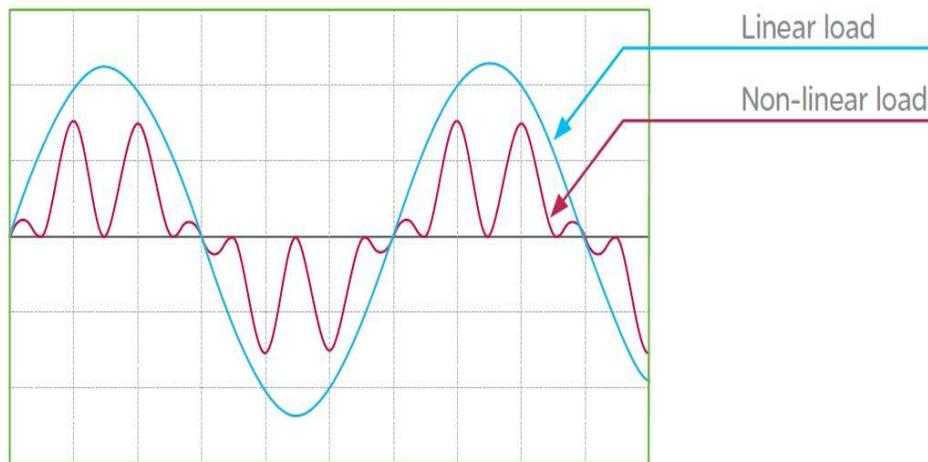
Figure 1: Linear and non-linear loads waveform (Schnieder, 2008)
