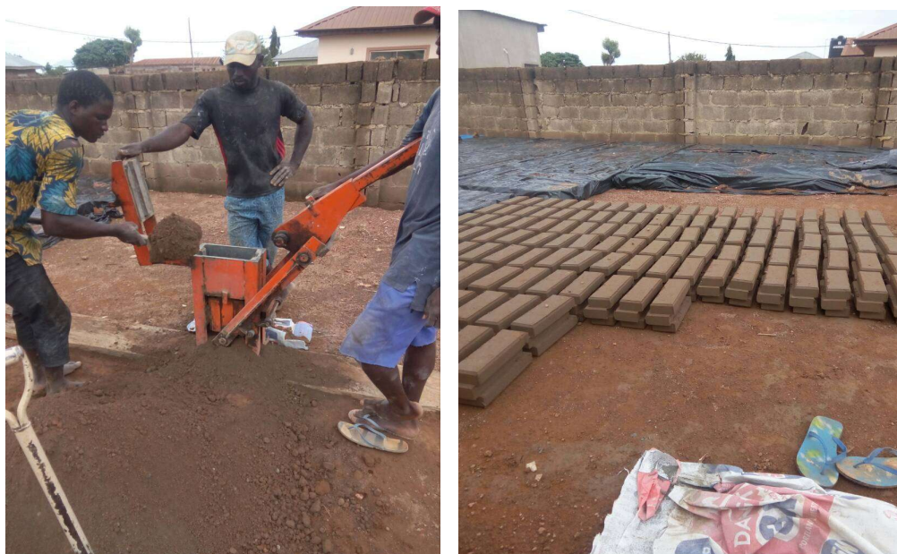
Figure 1: Earthen materials used for bricks
