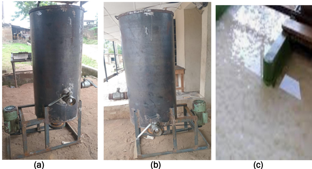
(a) (b) (c) Plate 2: (a) and (b) Plate of Pulper, (c) Slurry from Pulper Plate 2a, b and c showed the fabricated pulper and the pulp output.
