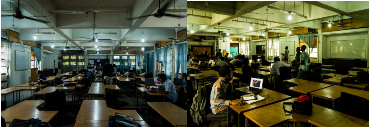
Plate1: Pictures showing the interior view of the architectural design studio for the Masters Class 2 with the individual work stations/movable seats, storage, interactive boards/projectors, fenestrations for natural ventilation and day lighting, means of mechanical ventilation, light fittings to enhance lighting in the studio, sufficient head room. .
