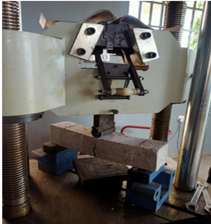
Plate 2: Beam Deformation after load application
