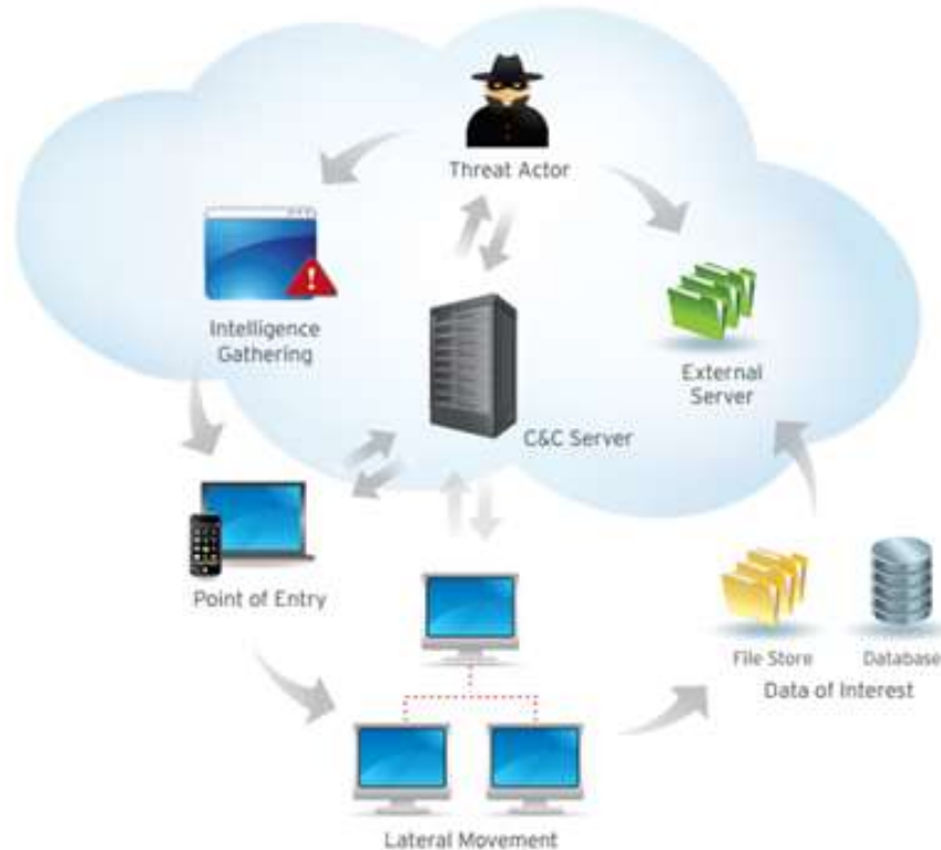
Figure 1: Anatomy of an APT attack (Anatomy of an APT Attack: (Source: Step by Step Approach, 2021)
