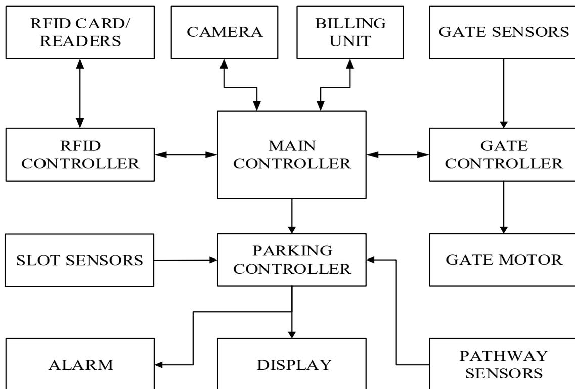
Figure 2: Block Diagram showing interconnection of various units
