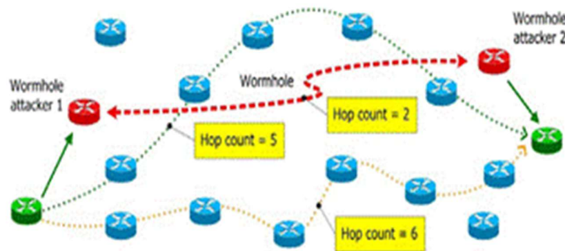
Figure 3: An out of bound (Hidden) Wormhole Attack launched through high powered transmission in MANETs
