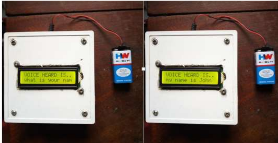
Fig. 7: The System Output During Testing
