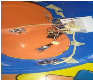
Fig 23: The devices are connected and placed in their compartments provided. The wires are well labeled.
