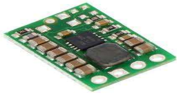
Fig 29: The 3.3V voltage Regulator
