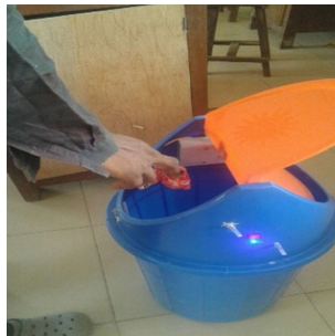
Fig 26: Trash Can opened at the closest proximity of 20cm at 150° inclination
