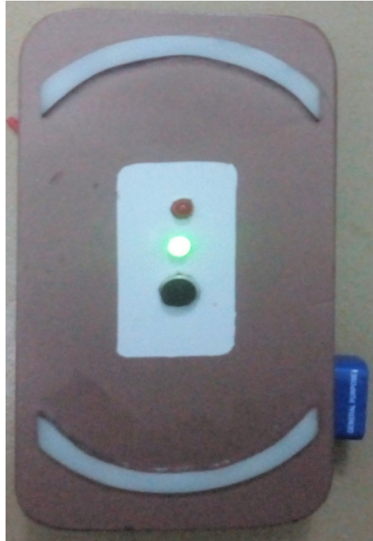
Fig 5: When the device senses the second clap
