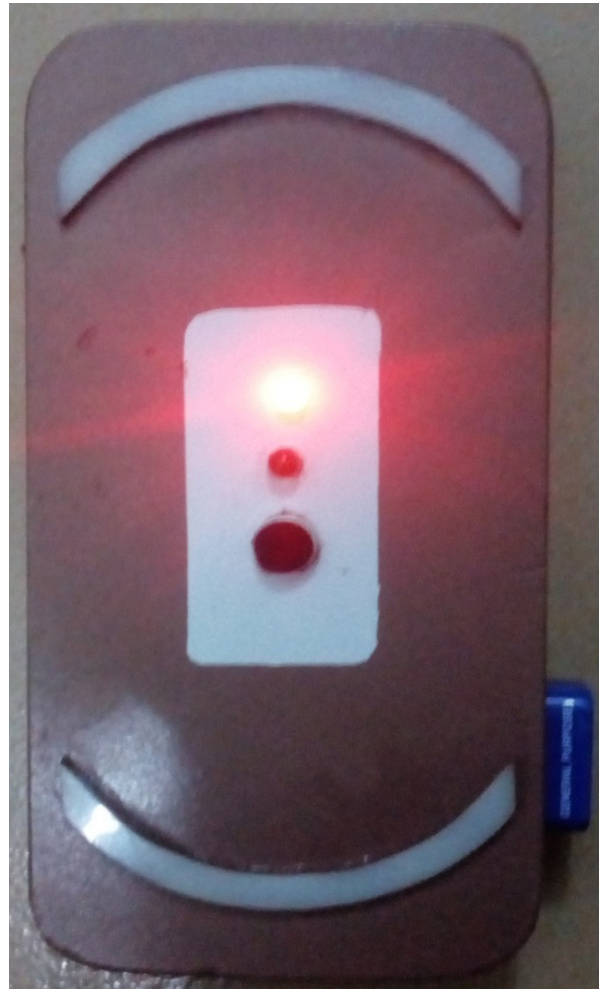
Fig 4: When the device senses the first clap (red LED turns ON)
