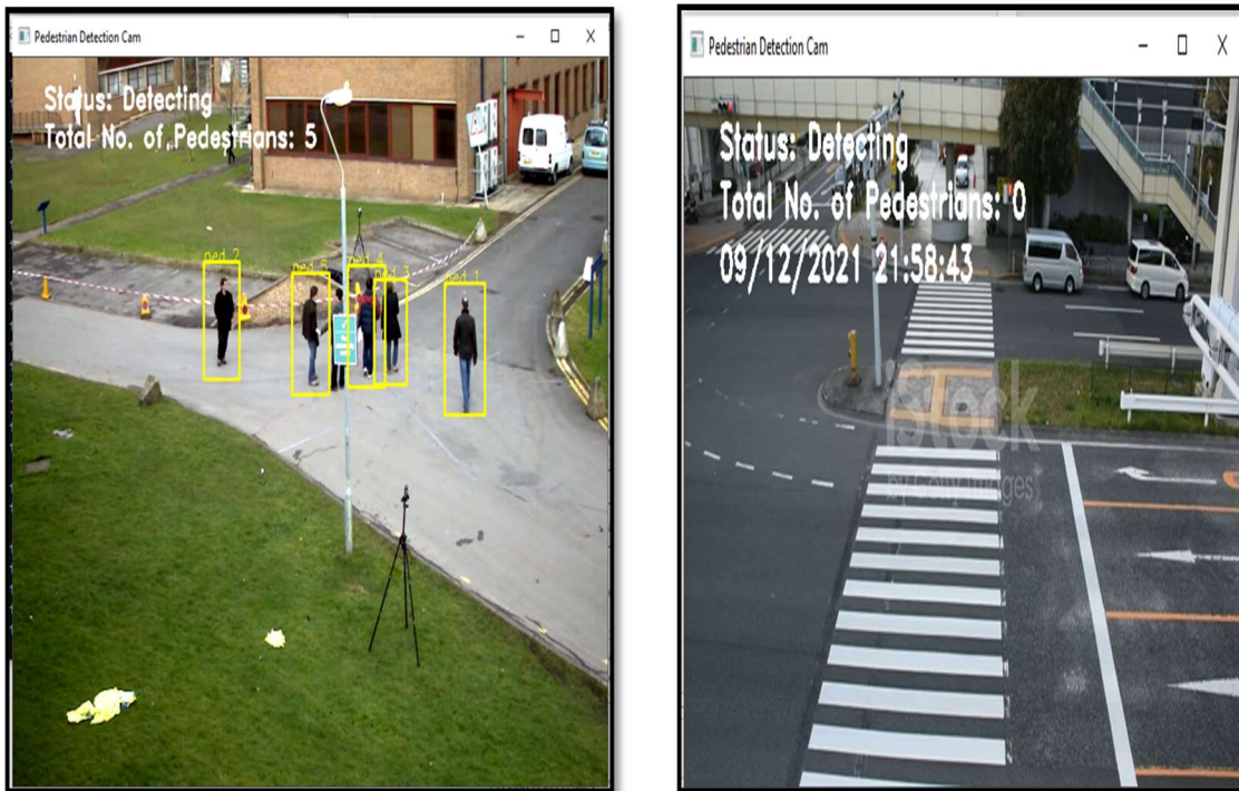
Fig. 2: Detection results using the pre-trained model acquired from the Haar Cascade Classifier
