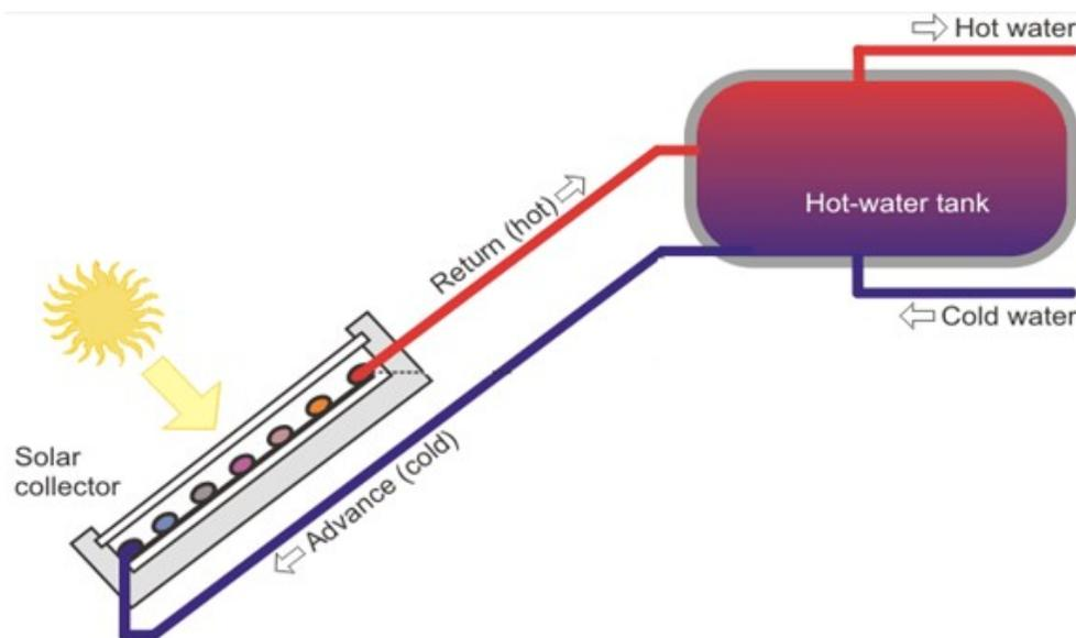
**Figure 1: The Schematic Diagram of a Thermosyphon solar heating system [6]**
