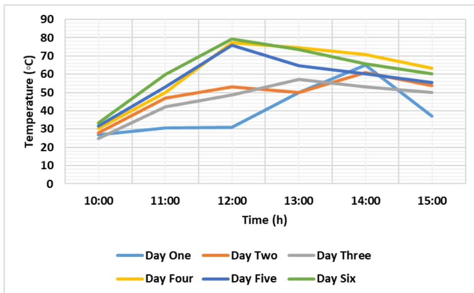
**Figure 5 Outlet temperature for the six days of testing**
