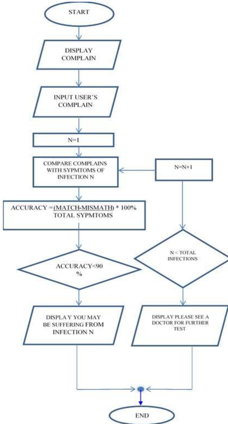
Fig.3.4: The Diagnose Process Flowchart
