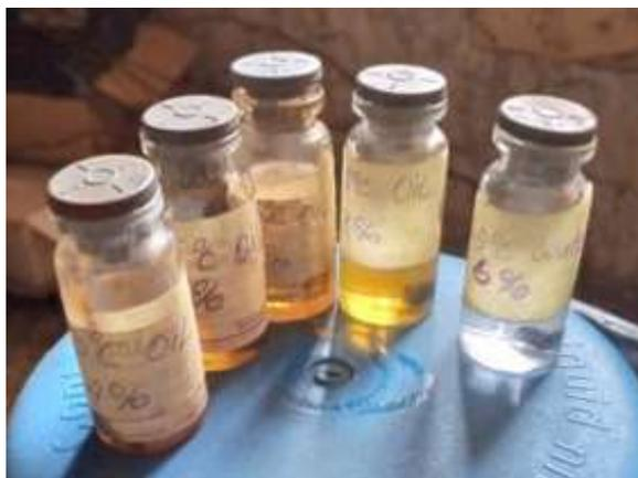
**Figure 4: Samples undergoing 6hours cold water, and oil thickness swelling tests and used for cold water and oil absorption test by TGA.**
