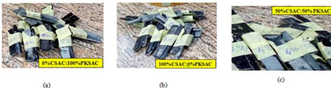
Figure 2: Epoxy/activated carbon composite samples.
