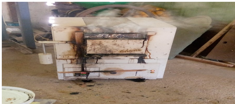
Plate 2: Corn-Cob calcined at 600°C at 4-5hrs (The temperature of the furnace was maintained between 625-650°C for about 4-5hours).
