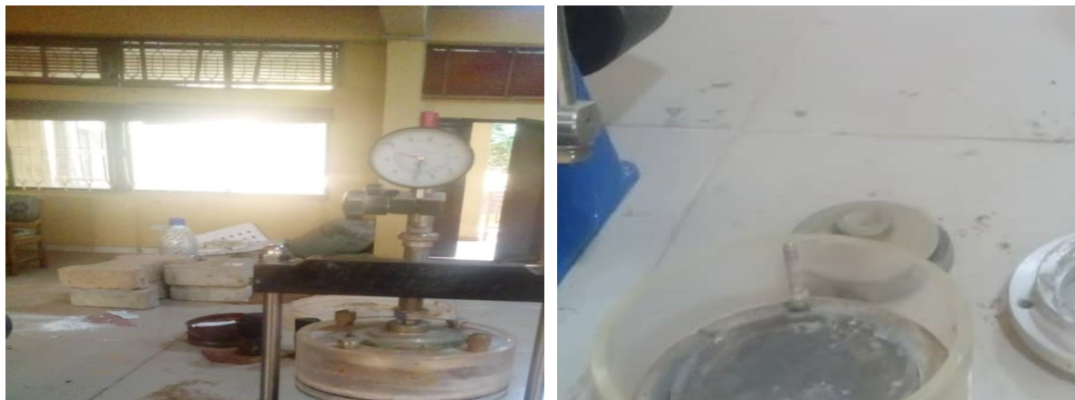
Plate 4: An Oedometer apparatus set-up (Consolidometer test)
