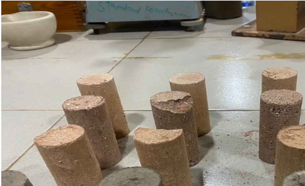
Plate 2: Unconfined compressive strength test specimens (50mm x 100mm), prepared and extruded from a cylindrical mold
