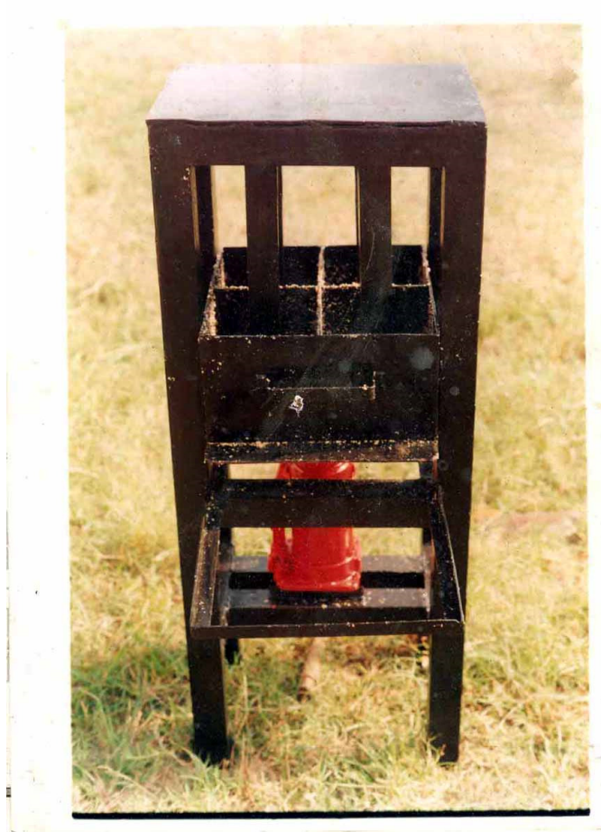
Plate 3:- A Prototype Briquetting Machine
