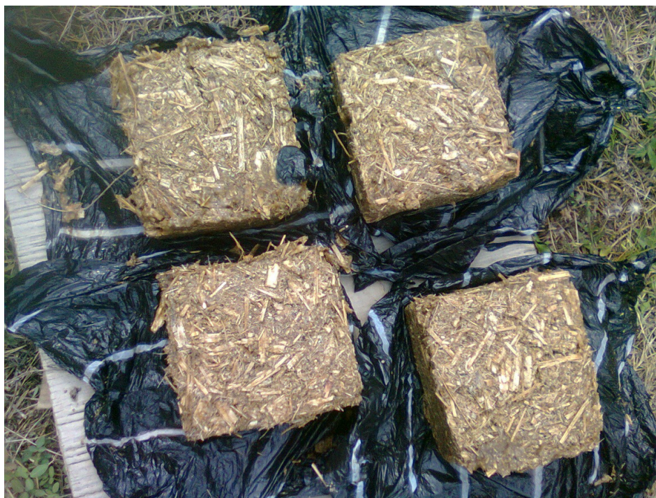
Plate 4:- Briquettes produced from Corn Stalk
