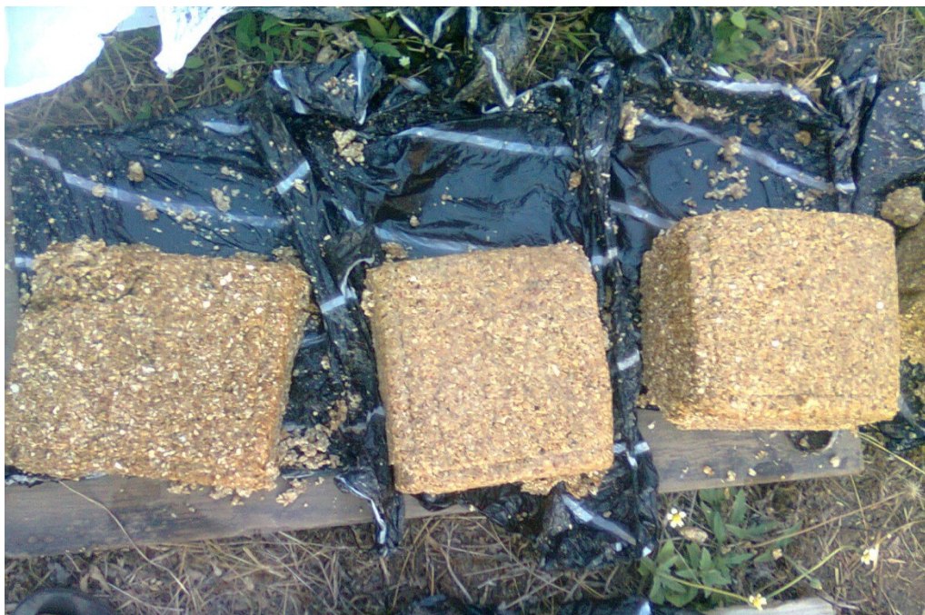
Plate 5. Briquettes from corncob residue
