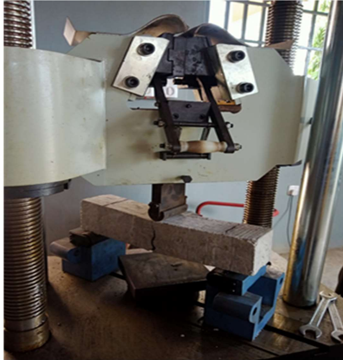
Plate 2: Beam Deformation after load application
