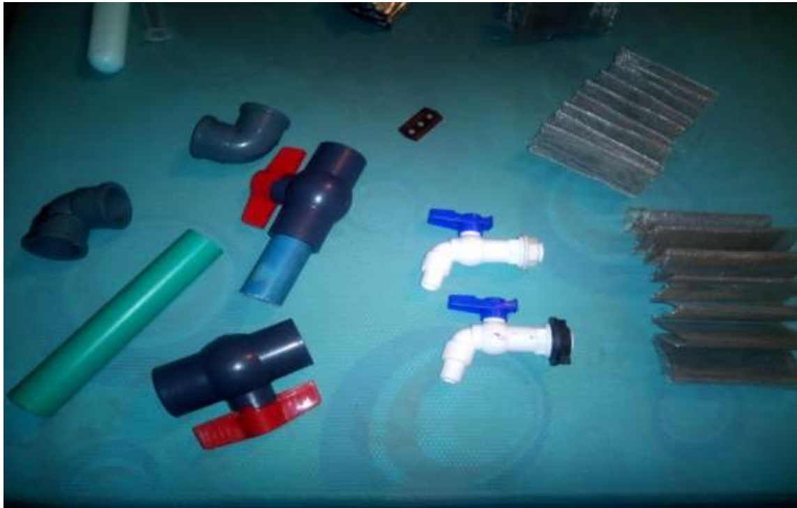
Fig. 4: PVC pipe, elbow joint, air valve, tap head and excess stainless steel wire mesh
