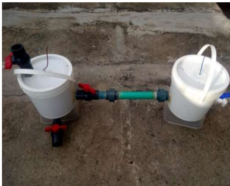
Fig. 7: Complete assembly of continuous flow MFC setup.
