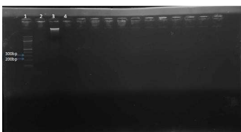
Figure 1: PCR gel electrophoresis profile for the confirmation of virulence gene in Brevibacterium linens
