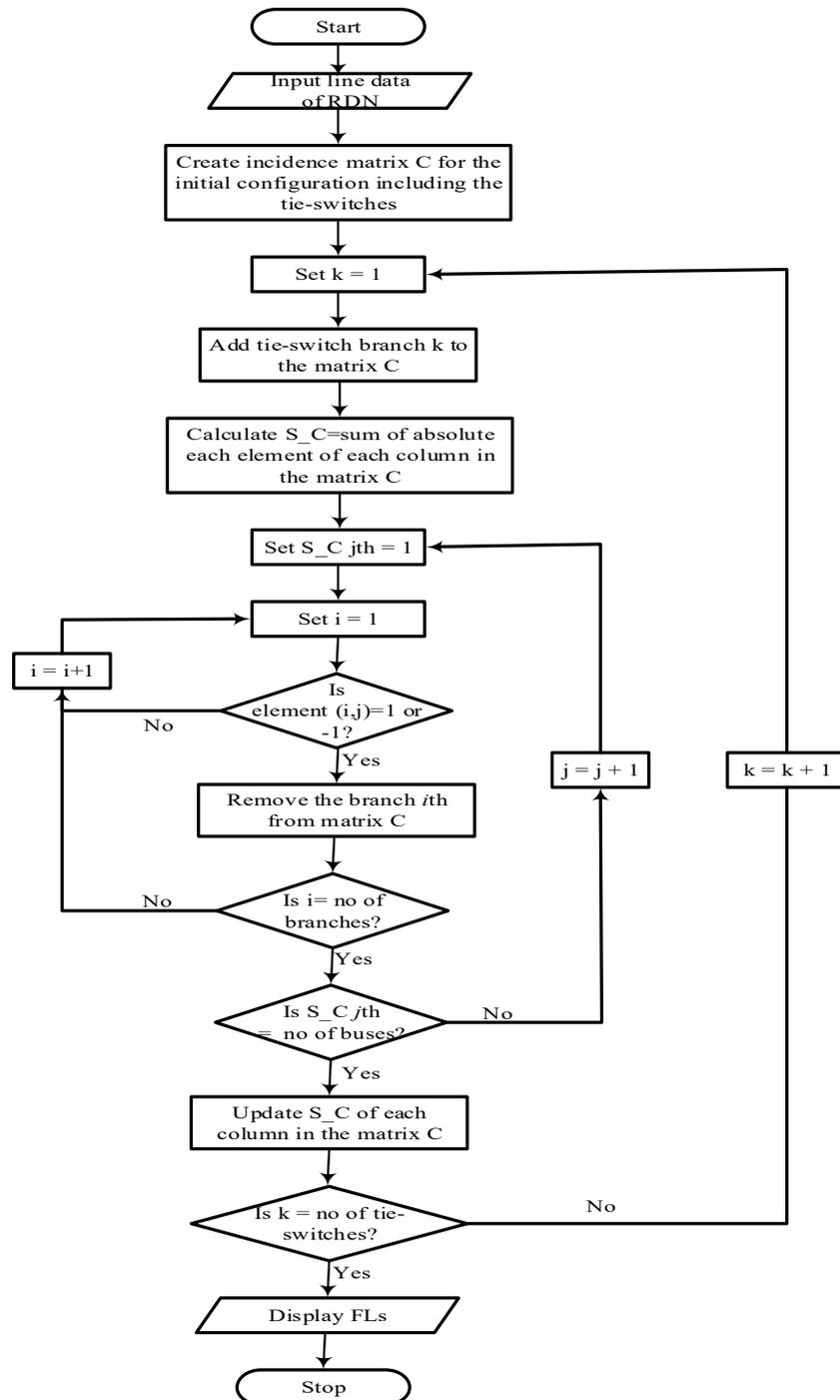
Figure 3. Flowchart for finding fundamental loops (FLs) of any RDN
