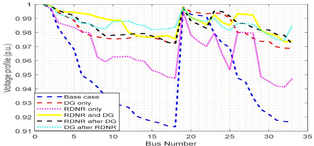
Figure 5. Voltage profile of events 1 - 6 for 33-bus RDN
