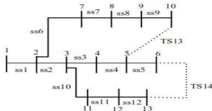
Figure 1. A simple sample of 13-bus RDN
