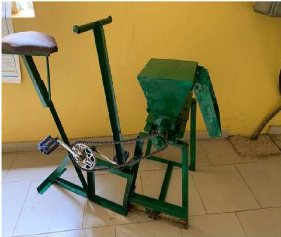
Fig. 6: Fabricated Pedal-Powered Locust Bean Dehulling Machine
